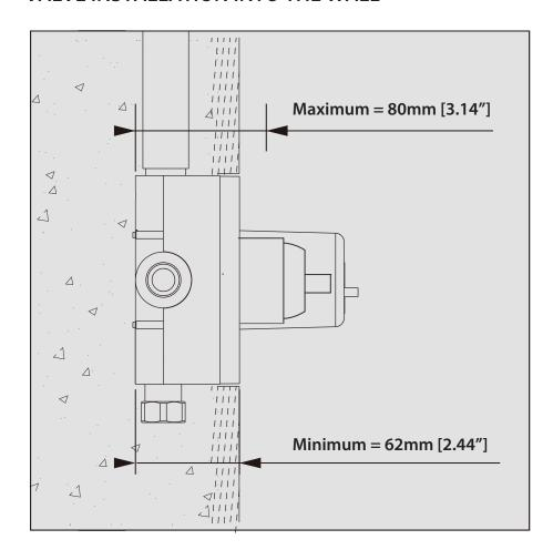
Install a crossbeam at the location where the valve will be installed. The distance between back of the valve to the finished tile surface should be between 2.44" and 3.14 inches.
